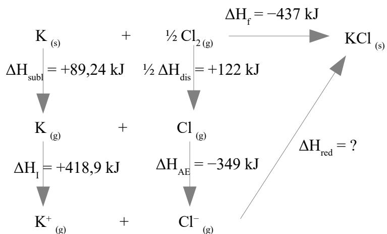
$$\Delta H_f = \Delta H_{\text{subl}} + \frac{1}{2} \Delta H_{\text{dis}} + \Delta H_I + \Delta H_{\text{AE}} + \Delta H_{\text{red}}$$
